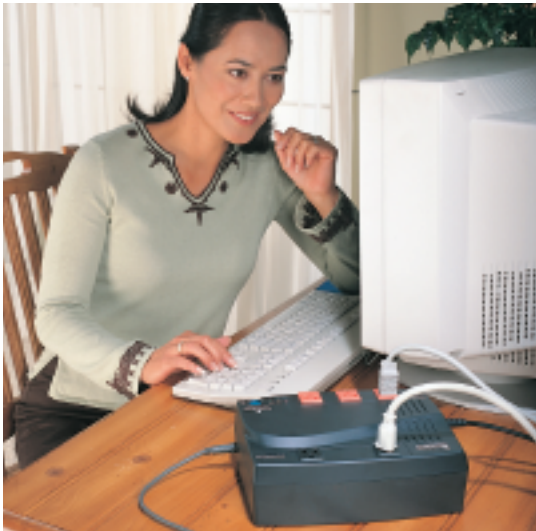
USB port offers communication to shut down if an outage ever exceeds battery capacity.
